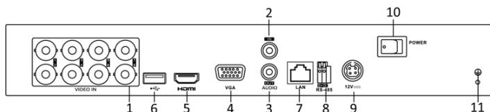
Figure 1. 6 Rear Panel of 720P Series
