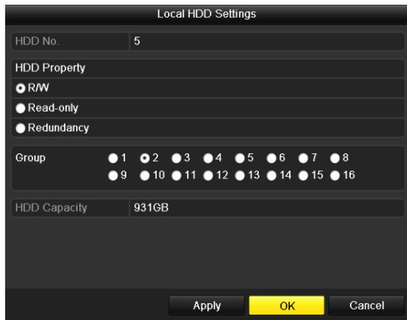
Figure 10. 15 Local HDD Settings Interface
