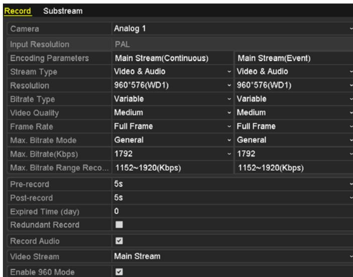
Figure 5.3 Record Encoding
