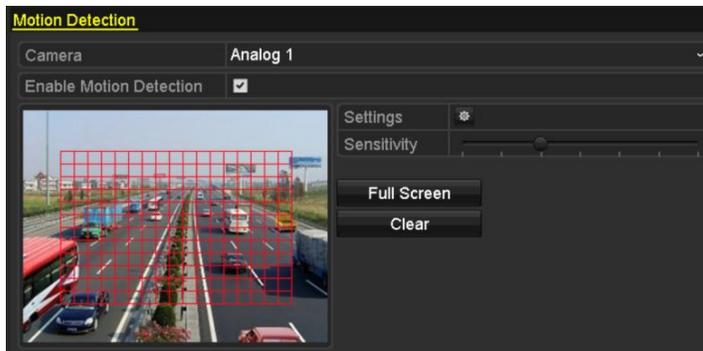
Figure 5.13 Motion Detection- Mask
