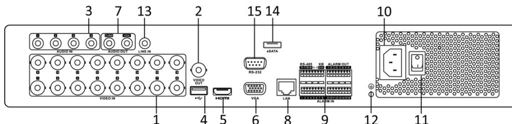
Figure 1. 7 Rear Panel of 1080P 1.5U Chassis Series
