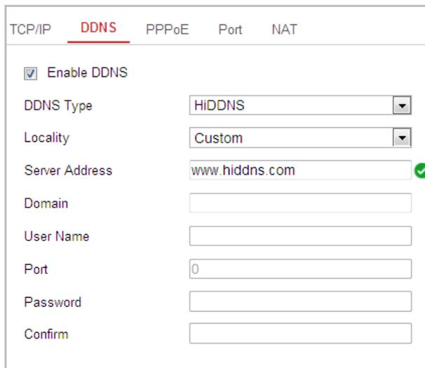
The screenshot shows the 'DDNS' tab of a settings form. It includes a checkbox for 'Enable DDNS' which is checked. Below it is a dropdown menu for 'DDNS Type' set to 'HiDDNS'. The 'Locality' dropdown is set to 'Custom'. The 'Server Address' field contains 'www.hiddns.com' and has a green checkmark to its right. Other fields include 'Domain', 'User Name', 'Port' (set to 0), 'Password', and 'Confirm', all of which are currently empty.
