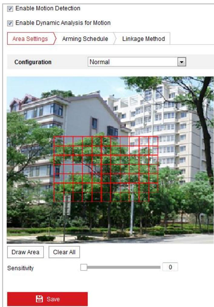
Figure 5-11 Motion Detection Settings-Normal
