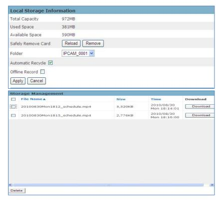
Click **Remove** to safely remove the storage device.
