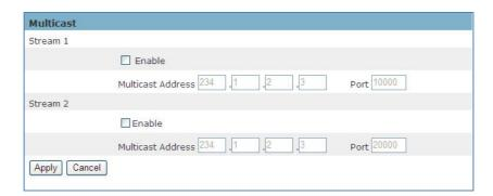
Multicast sends a video stream to the multicast group address and allows multiple clients to access the stream at the same time by requesting a copy from the multicast group address. Therefore, multicast can effectively save Internet bandwidth. The RTSP (Real-Time Streaming Protocol) controls the delivery of streaming media.
