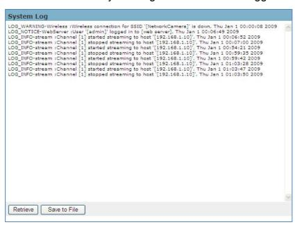
This page displays the system's log in chronological order. The system log is stored in the camera's buffer area and will be overwritten when the buffer area is full.
