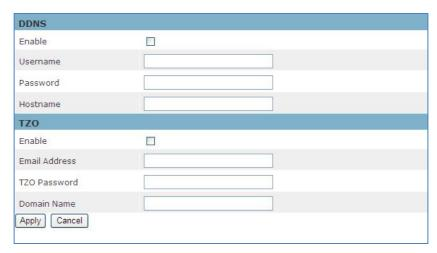
DynDNS - Enable the DynDNS to give the camera a fixed host and domain name. Refer to
