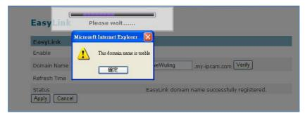
EasyLink has similar function with DDNS. User can create and use a memorized easily domain name after verifying successfully.
