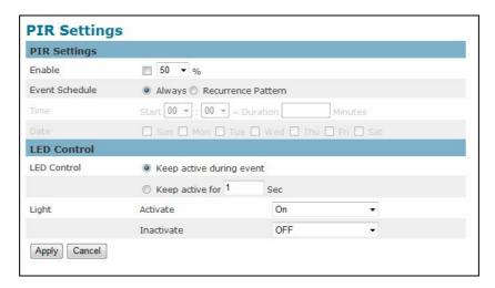
**PIR Settings** - The PIR (Passive Infra Red) sensor measures infrared light radiating from objects in its field of view. This can be used to detect a moving object, such as a person, in dimly lit areas.
