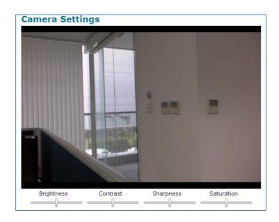
**Brightness -** Drag the slider bar to adjust the image brightness level from -5 to +5.
