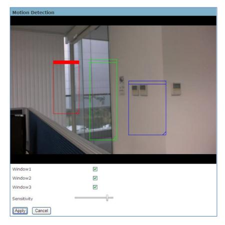
Use this setting to enable and define the motion detection windows. The user can define up to three areas on the live view window for motion detection.
