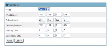
Static IP - Select this option to manually assign a static IP address to the camera. Enter
