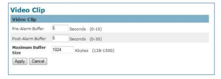
Video Clip can adjust the recording time and maximum buffer size before and after the event.
