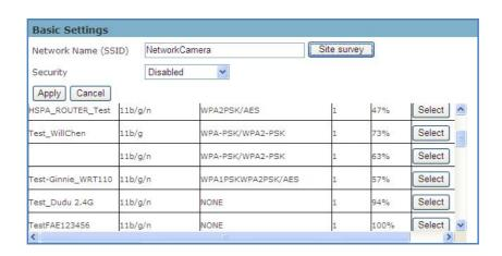
**Network Name (SSID)** - The Service Set Identifier (SSID) is the network name used to identify the wireless signal emitted from a wireless camera. It is case-sensitive and can be up to 32 characters long.
