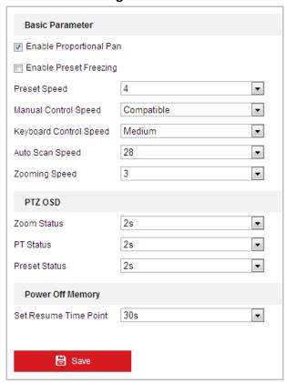
Figure 5-29 Basic PTZ Configuration Interface
