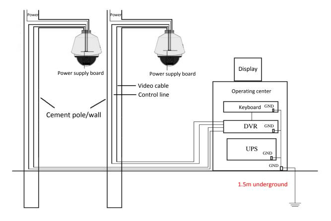
Figure A.3.2 Grounding in Cement Pole/Wall Installation
