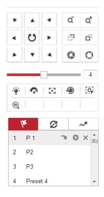
Figure 4-5 PTZ Control Panel
