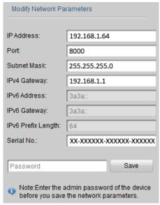
Figure A.1.2 Modify Network Parameters
