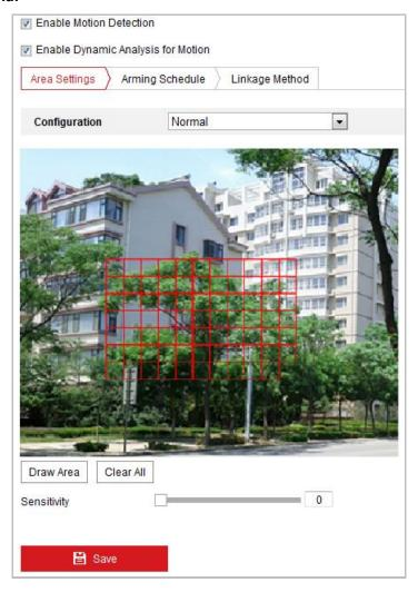
Figure 5-11 Motion Detection Settings-Normal
