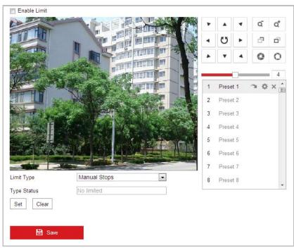
Figure 5-30 Configure the PTZ Limit
