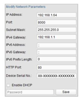
Figure 2-5 Modify the IP Address
