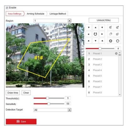
Figure 5-25 Configuring Intrusion Area
