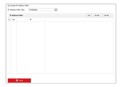
Figure 6-52 IP Address Filter
