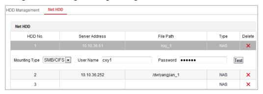
Figure 5-7 Select Net HDD Type
