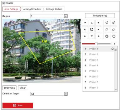
Figure 5-28 Configuring Region Exiting Detection
