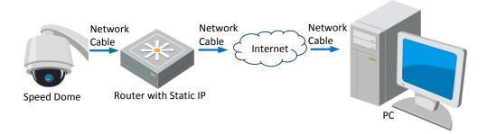
Figure 2-10 Accessing the Speed Dome through Router with Static IP
