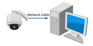
Figure 2-1 Connecting Directly
