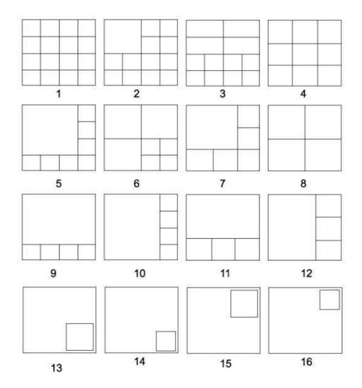
For 16 channel multiplexer, the sequence of 16 different displaying modes are shown as above. It allows selecting a favorite mode for monitoring by pressing the MODE button, if necessary.
