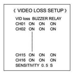
When video loss function is set to 'ON', the unit will respond to a loss of camera video as an alarm status. If it is set to 'OFF', the unit will not detect the loss of the camera images, even if a video loss occurs.
