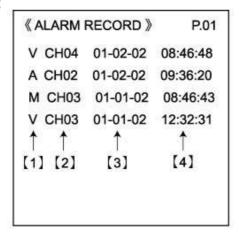
This menu is where you can find out when the alarm sensor, the loss of camera image and motion detection were activated. 100 records are separated in 10 pages and the last hundred alarm events are recorded, with the oldest one being deleted when triggered again.
