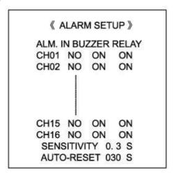
There are two types of N.C. (normally closed) and N.O. (normally open) in the alarm sensor. When the sensor type setting on the screen doesn't correspond with current sensor status, a "?" mark will appear between sensor status and sensor type, that means an error.
