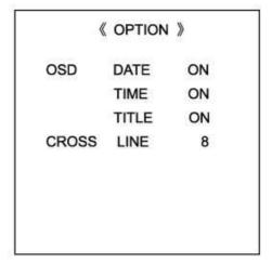
OSD DATE ON/OFF: It is an On/Off switch for the display of Date.
