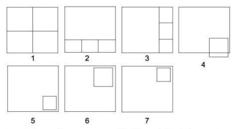
For 4 channel multiplexer, the sequence of 7 different displaying modes are shown as above. It allows selecting a favorite mode for monitoring by pressing the MODE button, if necessary.
