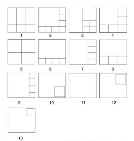
For 9 channel multiplexer, the sequence of 13 different displaying modes are shown as above. It allows selecting a favorite mode for monitoring by pressing the MODE button, if necessary.
