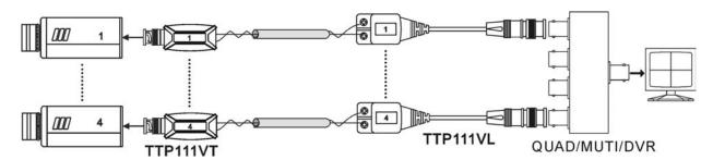
\* Used as Receiver, the HTA-TTP111VL compact size is perfect to connect with the image processor, which have multi BNC connections, as like Multiplexer, Quad, DVR ...etc.
