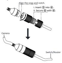
Figure 2-11 Water-proof Accessory Installation
