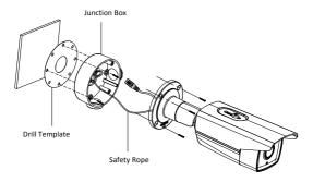
Figure 2-8 Installation with a Junction Box
