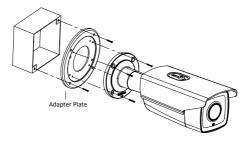
Figure 2-9 Installation with a Gang Box
