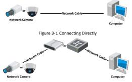
Figure 3-2 Connecting via a Switch or a Router
