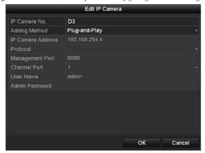
Figure 2. 23 Edit IP Camera Interface - Plug-and-Play
