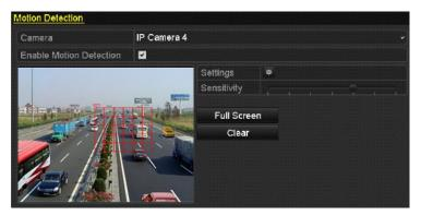
Figure 5. 10 Motion Detection- Mask
