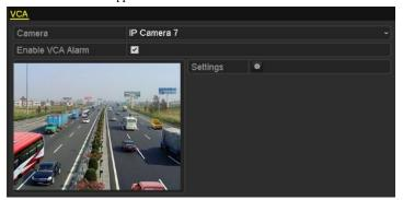
Figure 8. 13 VCA Alarm Setting Interface
