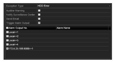
Figure 10. 23 Configure HDD Error Alarm
