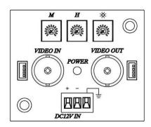
When using multi amplifier, a jumper is needed to extend power. (Max of 3 units by DC12V/500mA Power adapter package include )
